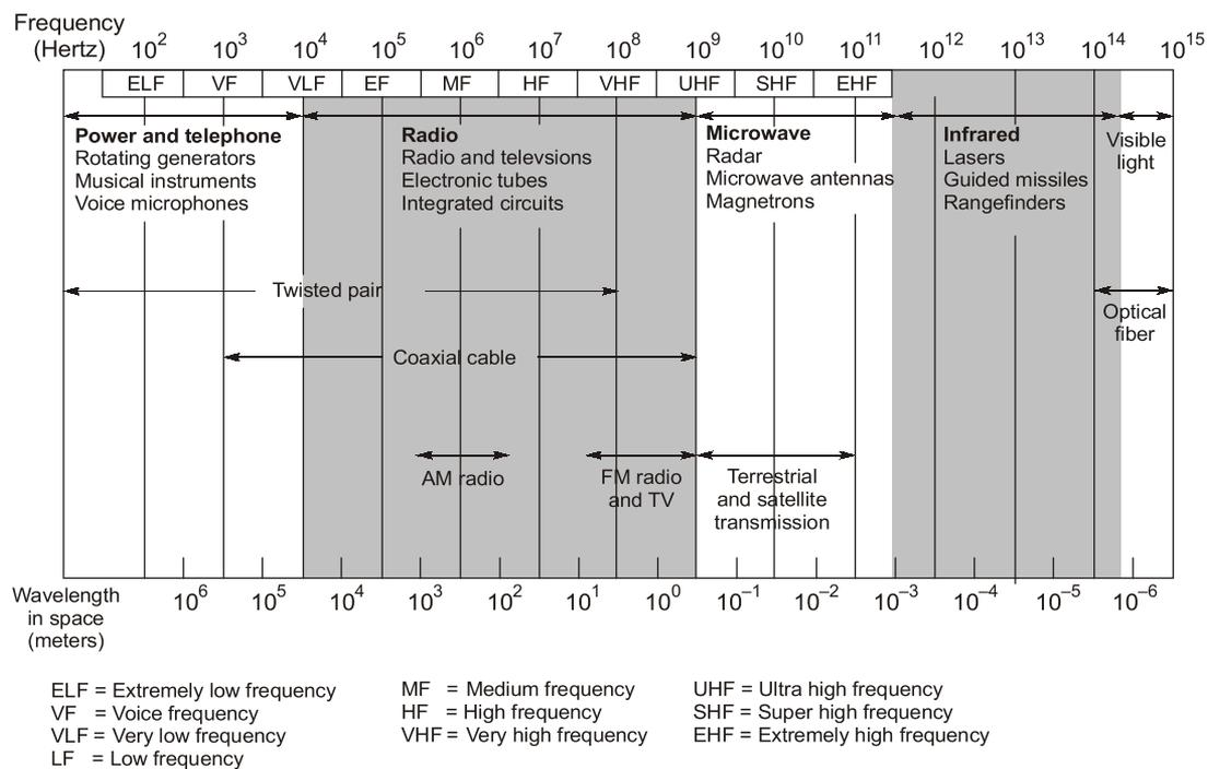
**Figure: Electromagnetic spectrum for telecommunication**
